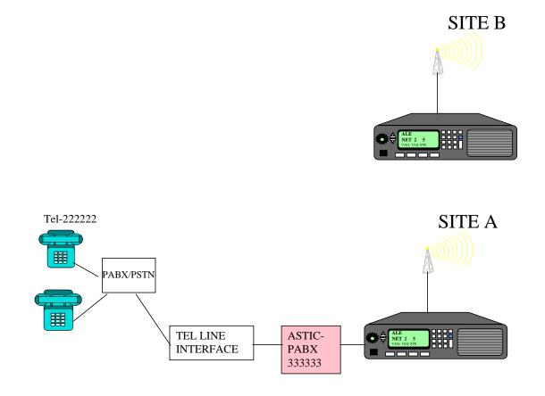
A Telephone (number 222222) calling remote Micom-2E radio at site B.
